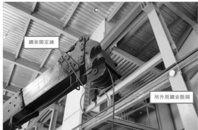
肇災積載型卡車起重機之吊桿上未裝設過捲預防裝置
